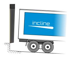
Bevelled cushions reduce the opening of the loading bay, thus guaranteeing proper sealing.
